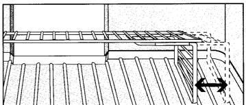
The **Twin Expandable Freezer Shelf** allows for increased freezer storage capacity by adding another shelf. To accommodate for varying frozen food loads, the height of the shelves can be adjusted. The lower shelf has expandable width capabilities (as described above) so an area for taller items can be created.
